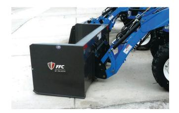
FFC also features **Compact Tractor Snow Pushes** designed to mount on tractor frontend loaders with universal skid steer style mountings. Lift capacity of the loader should be less than 2,000 lbs. These snow pushes have side wearing skids and a rubber cutting edge.
