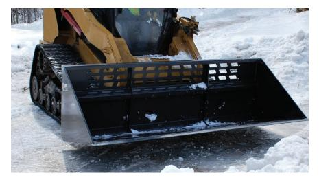
**Snow Buckets** move large volumes of snow or other loose materials efficiently. Equipped with a cut out back plate for better visibility. Quickly attaches to all skid-steer, backhoe, utility loader and small wheel loader brands. Optional Bolt on edge available. For SSL, Compact Utility Loaders, Compact Wheel Loaders, and Backhoe Loaders
